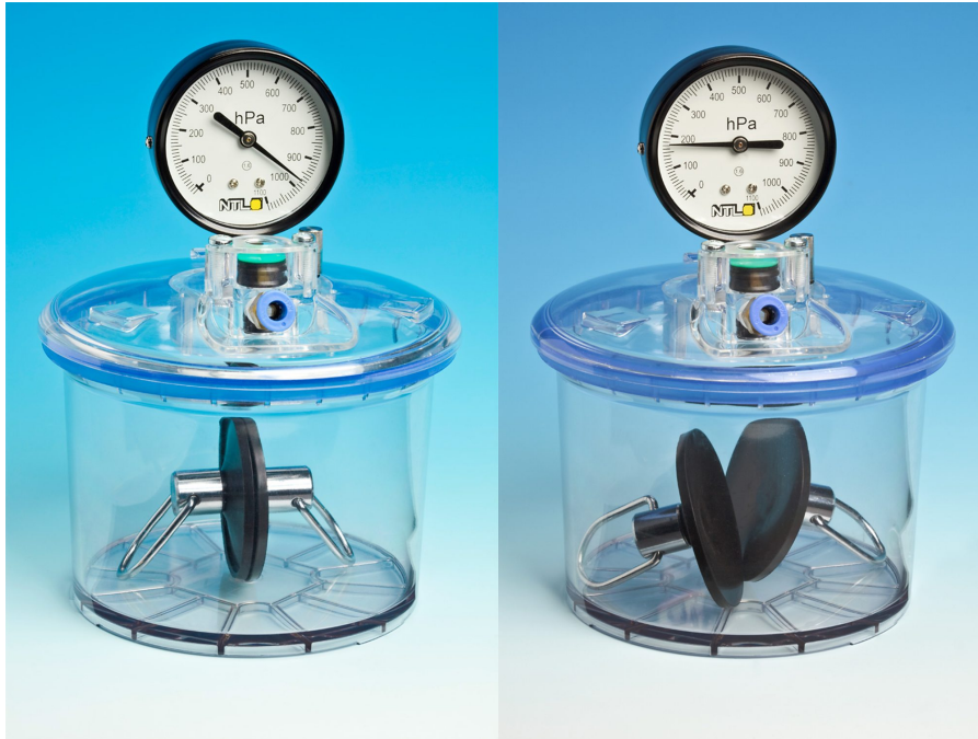
RUBBER SEALS BEING USED AS A DEMONSTRATION OF THE MAGDEBURG HEMISPHERES
